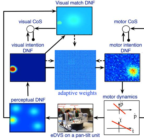
Fig. 1: The DNF learning architecture: the eDVS provides a visual input to the perceptual Dynamic Neural Field (DNF), which in its turn drives the visual intention DNF, and, through an adaptive mapping, the motor intention DNF. Visual and motor condition-of-satisfaction (CoS) nodes control the action-perception flow, and the visual match DNF detects moments, when the mapping should be updated.
