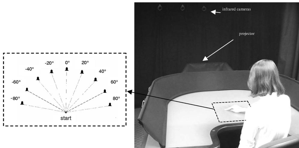
*Figure 4.* Apparatus used for spaceship task. Inset shows sample target locations relative to the starting point. Targets are projected onto the table from beneath and responses are recorded using an Optotrak movement analysis system. Note that the lights in the room are turned on for the photograph. During the experiment the lights were dimmed, and the table appeared black.
