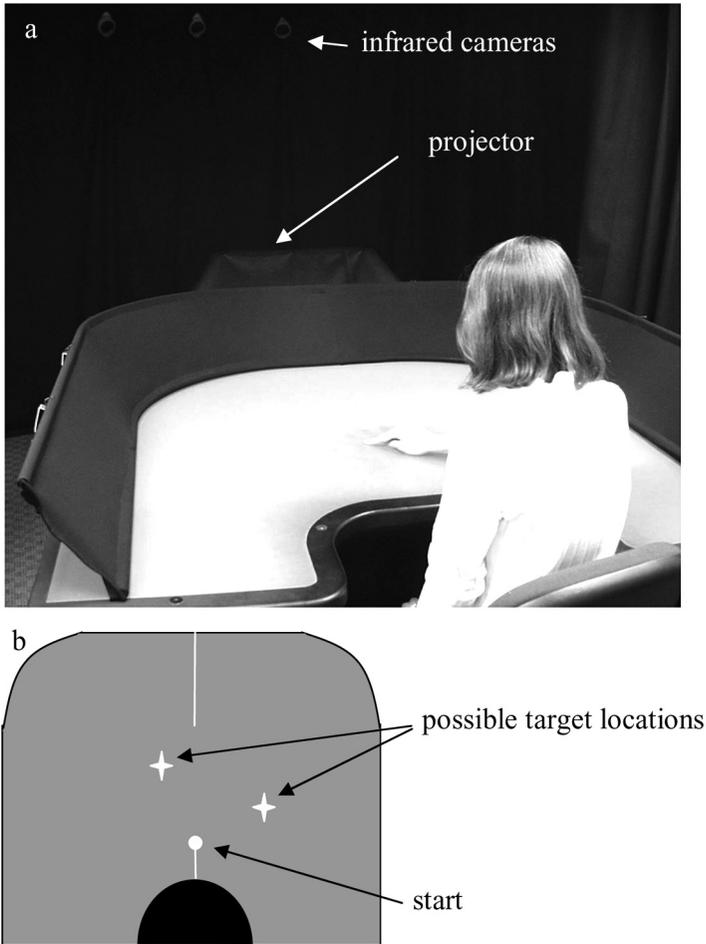
**FIGURE 4** Apparatus used for spaceship task (a). Targets are projected onto the table from beneath and responses are recorded using a motion tracking system. Note that the lights in the room were turned on for the photograph but were dimmed during the experiment so the table appeared black. Schematic shows the table top with the enhanced midline axis display and sample target locations relative to the starting point (b).
