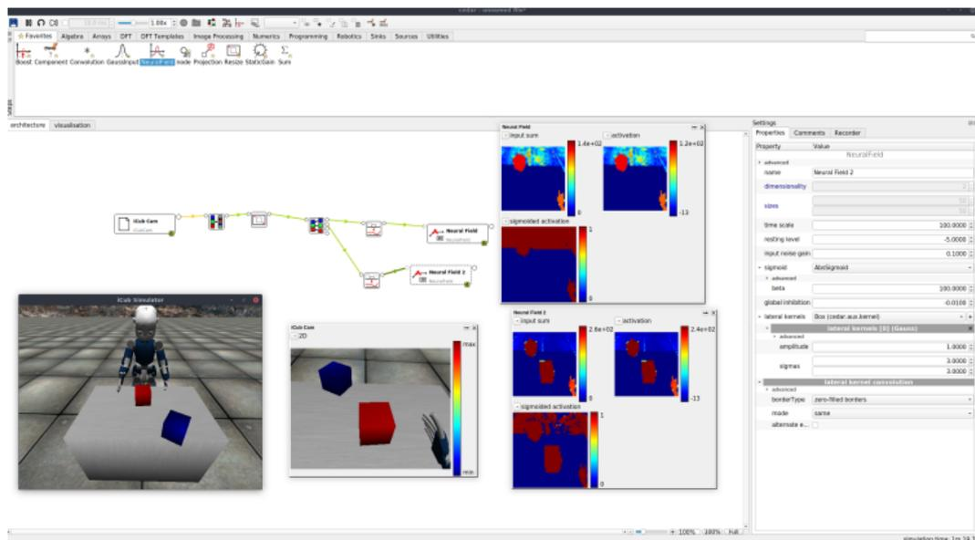
Plugins also available to control the iCub end-effector (left or right arm) from a 2D or 3D Neural Field.
