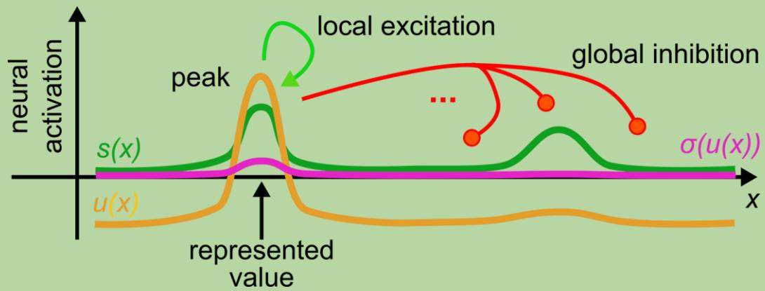
$$\begin{aligned}\tau \dot{u}(x, t) = & -u(x, t) + h + s(x, t) + \xi(x, t) \\ & + \int \omega(x - x') \sigma(u(x', t)) dx'\end{aligned}$$
